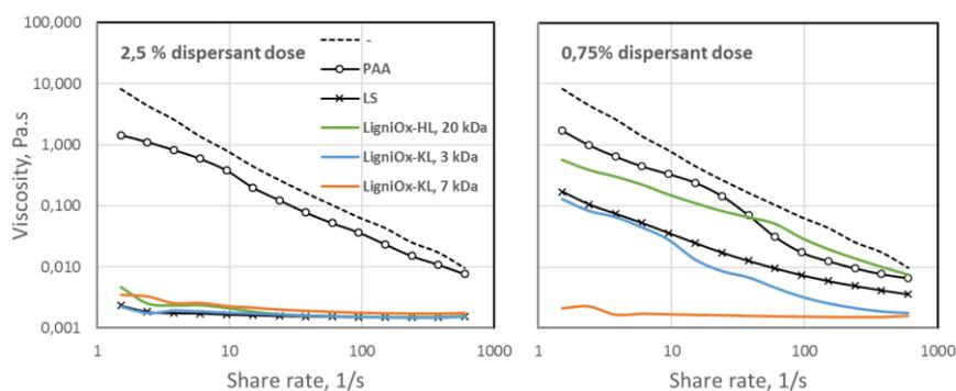
**Figure 3.** Viscosity of special carbon black dispersion with commercial dispersants (PAA, LS), kraft (LigniOx-KL 3 & 7 kDa) and hydrolysis lignin (LigniOx-HL 20 kDa) based LigniOx. Dosing 2,5 & 0,75% of carbon black.
