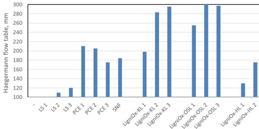
**Figure 1.** Haegermann flow in fresh mortar plasticized with commercial (super)plasticizer products (LS, PCE, SNF) and kraft, organosolv, and hydrolysis lignin based LigniOx. Dosing 0,6% (based on lignin content) of cement. Defoamer used.
